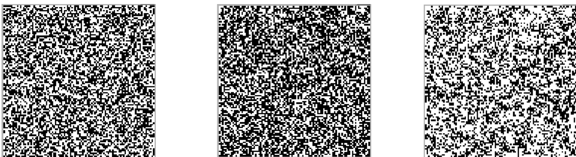
Figure 6. Left: snapshot of the grid during a normal trading period. The black cells are the buyers, while the white ones are the sellers. The parameters used in this simulation are \lambda = 1 , \kappa = 9 , and \mu = 2 \times 10^{10} . Center: bull market, where buyers predominate. Right: the same simulation during a crash
