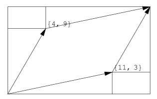
The total area of the rectangle is given by (a + c)(b + d) while the area of the parallelepiped can be found by subtraction of the small rectangles and triangles, thus  $(a + c)(b + d) - 2bc - 2*(\frac{1}{2}ab) - 2*(\frac{1}{2}cd) = ad - bc$ . This latter value is the determinant of the matrix.
