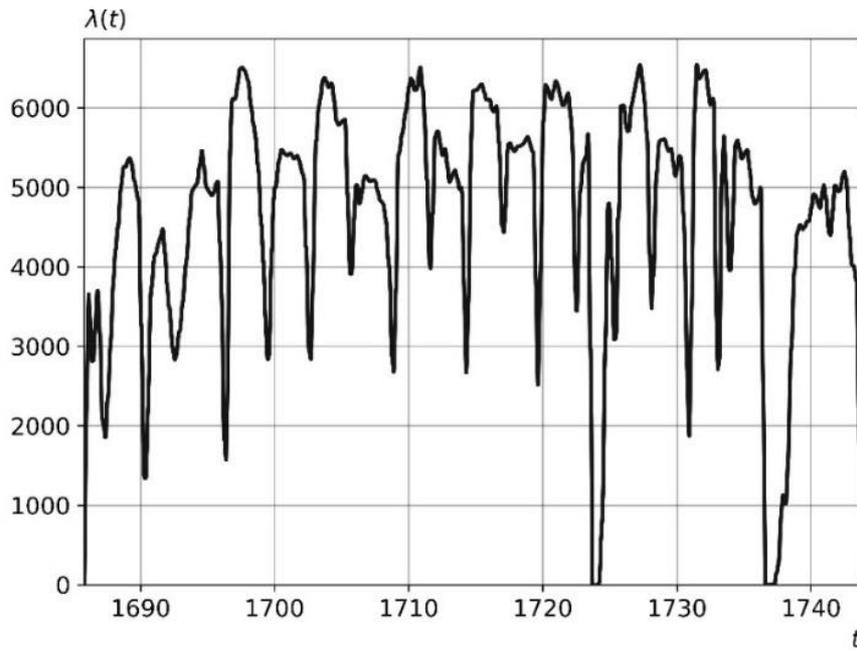
**Figure 1:** Actual volume capacity for the SRs 2000 bucket-wheel excavator recorded in the Belchatow surface lignite mine during the excavation of one terrace [29]
