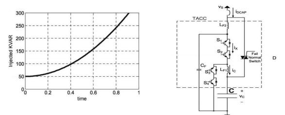
If the AC chopper is modulated with the cycle  $D = k_0$  at high frequency f, the equations  $V_c$  and  $I_x$  are obtained from the following equation:
