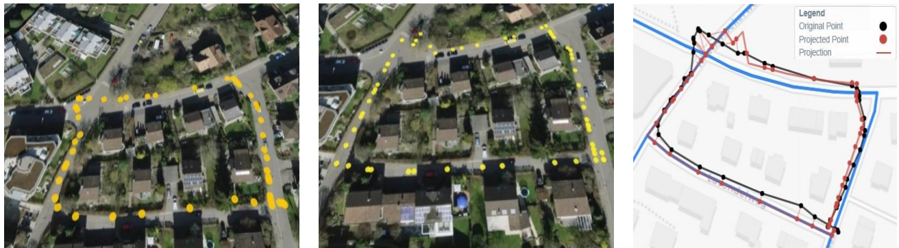
Fig 1 (a) Raw GPS data (b) Processed GPS data after using HMM (c) Original point i.e. raw GPS data and processed data with projection using available python package.
