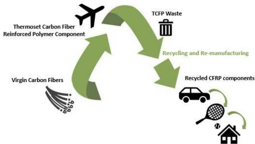
Figure 4 - Cascade downcycling of Thermoset Carbon Fiber Reinforced Polymers Components from the aviation industry
