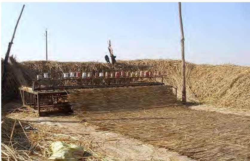
Photograph 15 – Weaving loom for reed mats at Wuliangsu Hai Lake, Inner Mongolia ( J. F. Köbbing, 10 September 2012 ).
