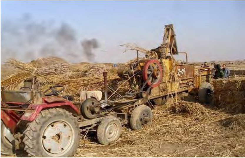
Photograph 17 – Loading reed onto a pressing machine for bales at Wuliangshuai Lake, Inner Mongolia (J. F. Köbbing, 3 September 2012).
