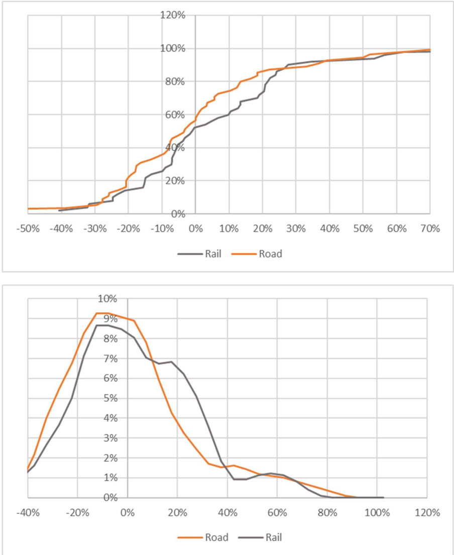
Figure 6. Distribution of cost changes from “ready to start” to final cost. Top diagram is cumulative distribution (raw data), bottom figure is density function (smoothed with a kernel estimator).
