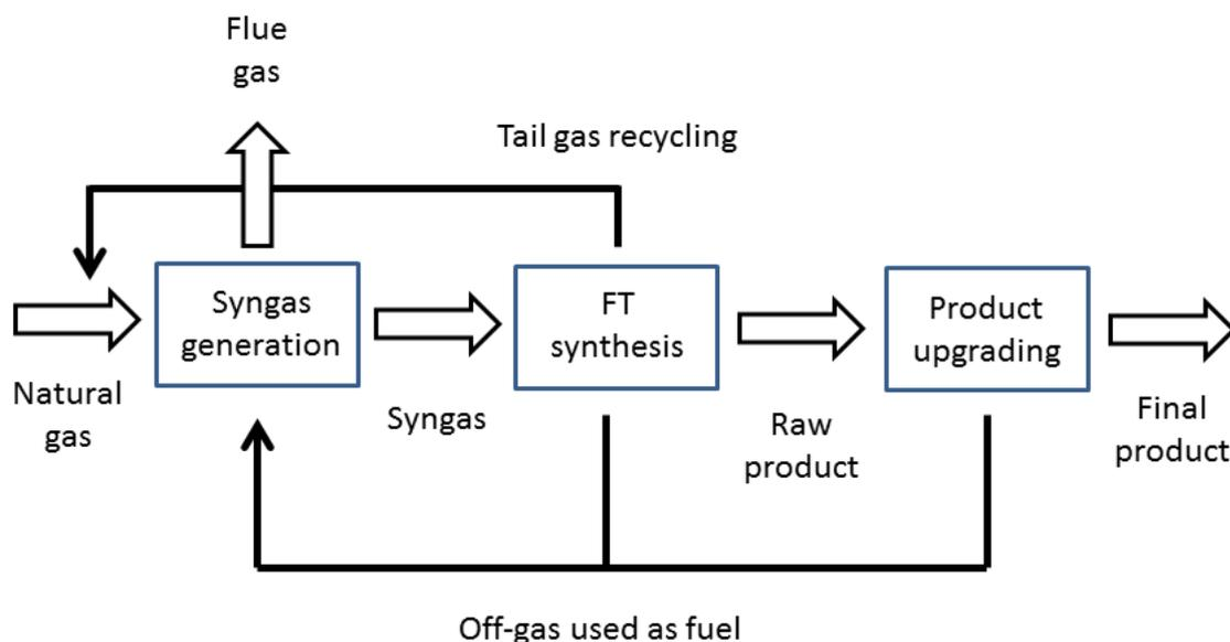
**Figure 1.** Simplified process chain for a GTL complex.
