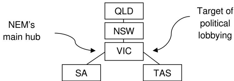
However, NEMLink provides a solution to the maladaptation in Victoria exacerbated by Victoria's position as the main hub in the NEM. Figure 6-8 shows the topology of NEMLink. Garnaut (2011, p. 32) discusses NEMLink (AEMO 2010b) as providing a truly national grid by adding interconnectors between SA and QLD and between SA and TAS. The current grid topology in
