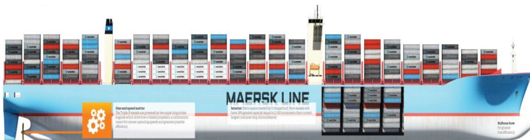
Figure 21. 2 The Triple-E engines consume 37% less fuel oil and emit 37% less CO 2 per container. The ship itself is 95% recyclable. Triple-E (EEE) stands for E conomy of scale, E nergy efficient and E nvironmentally improved vessel. Source: Maersk
