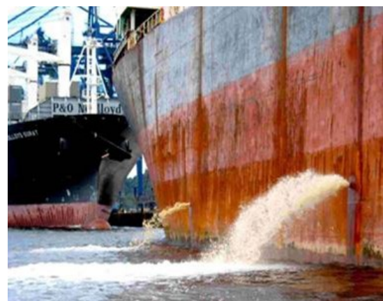
Figure 10. Ballast water is used to stabilize the ship as it receives or tranship cargo.
