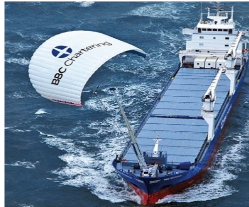
Figure 23. SkySails®. This technology promises to revolutionize the maritime industry.
