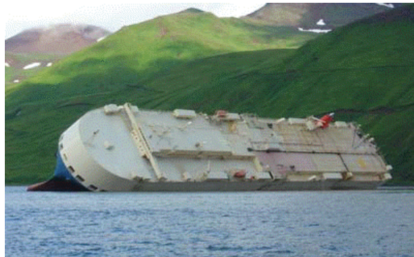
Figure 12. The "Cougar Ace" turned down due to stability problems with the ballast on his way to Vancouver in 2006.
