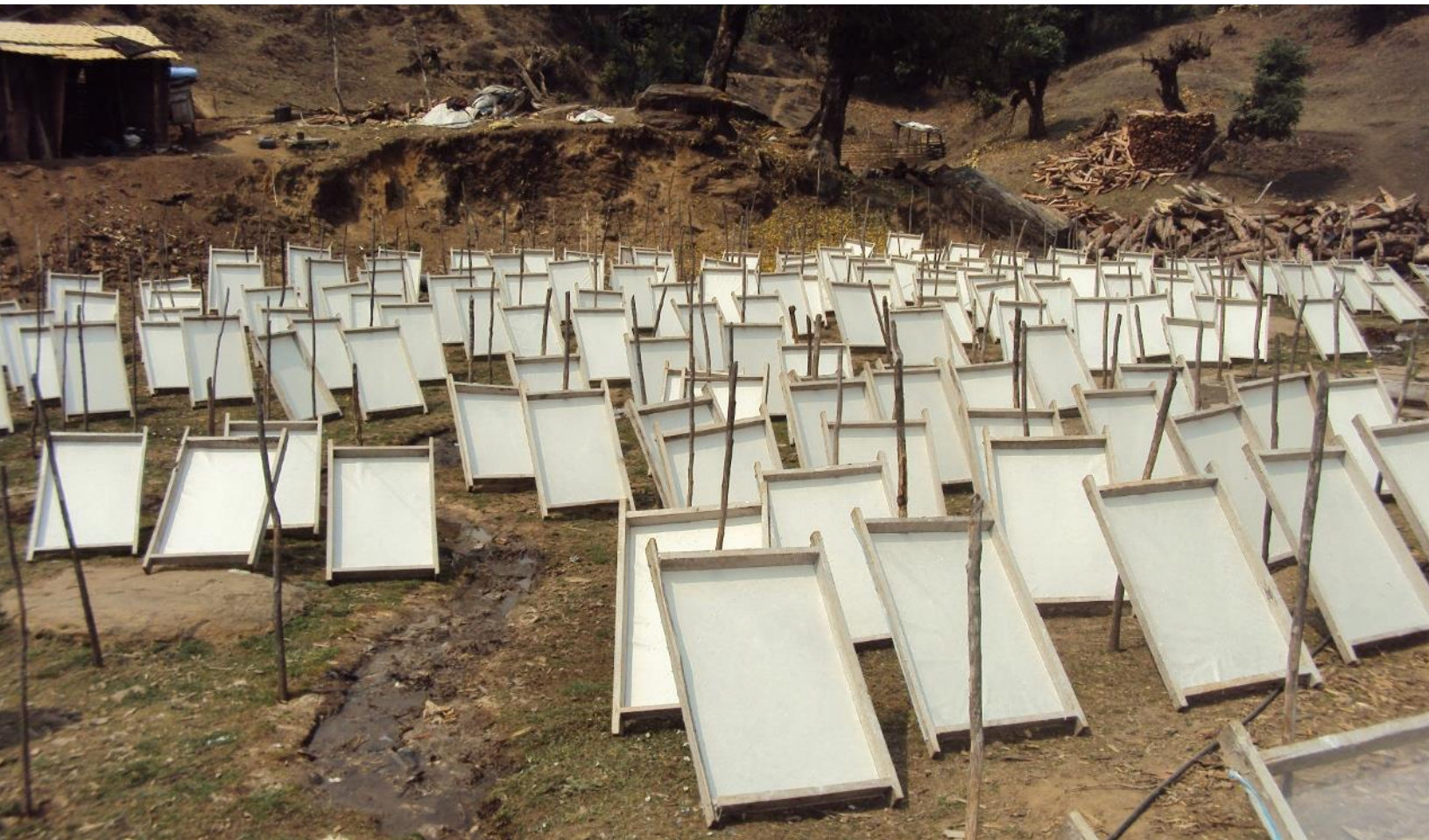
Figure 4: Traditional handmade Lokta paper being dried. © Pitambar Shrestha, LI-BIRD
