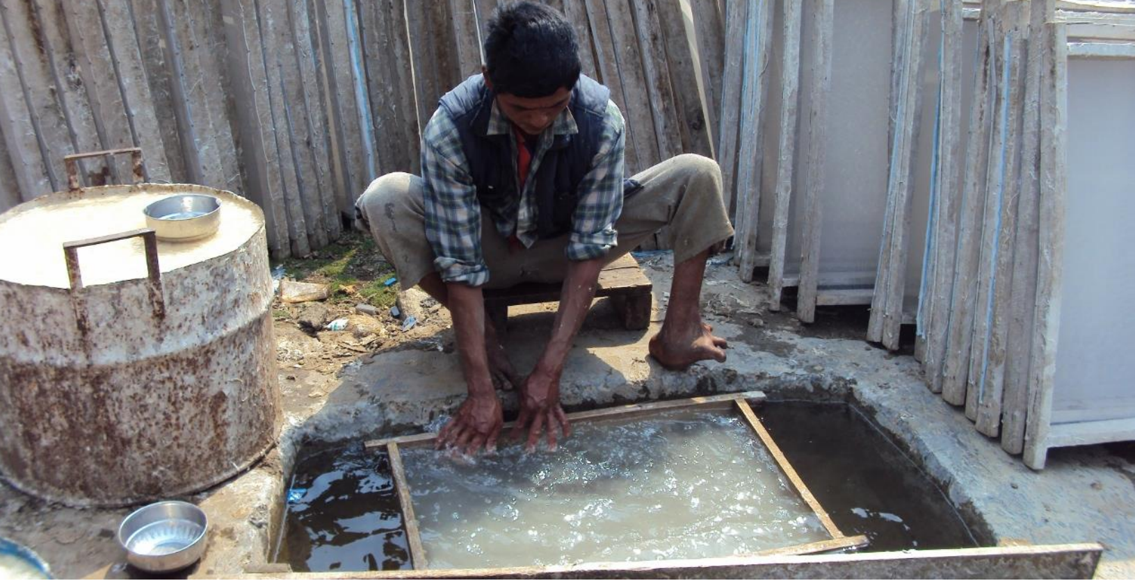
Figure 3: Preparing traditional handmade lokta paper in Tamaphok. © Pitambar Shrestha, LI-BIRD
