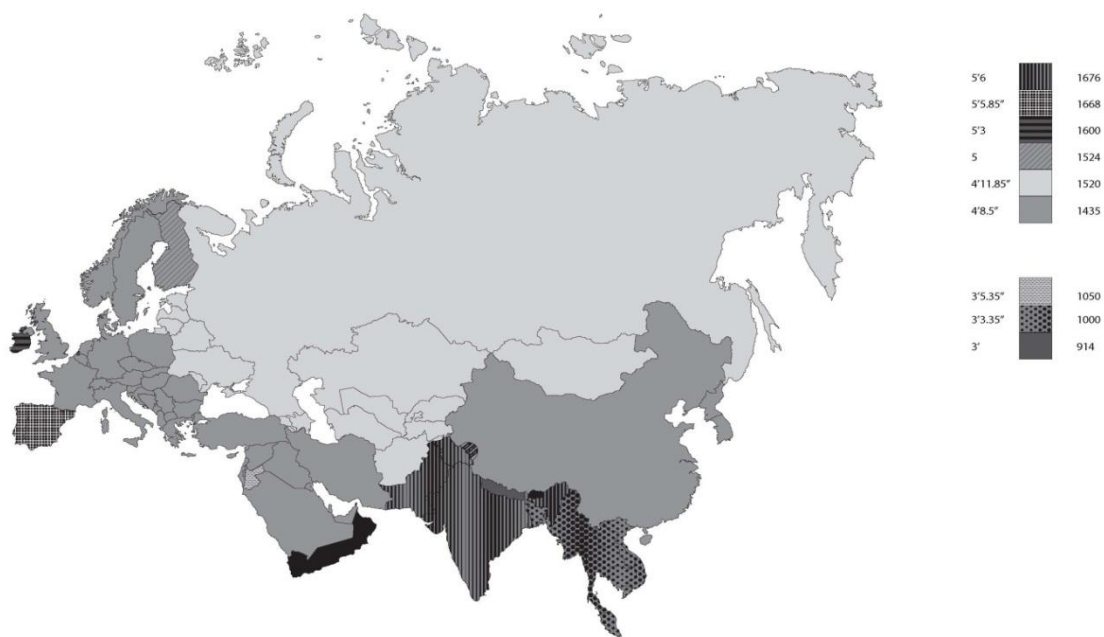
Figure 7 - Eight types of railway gauges used in Eurasia
