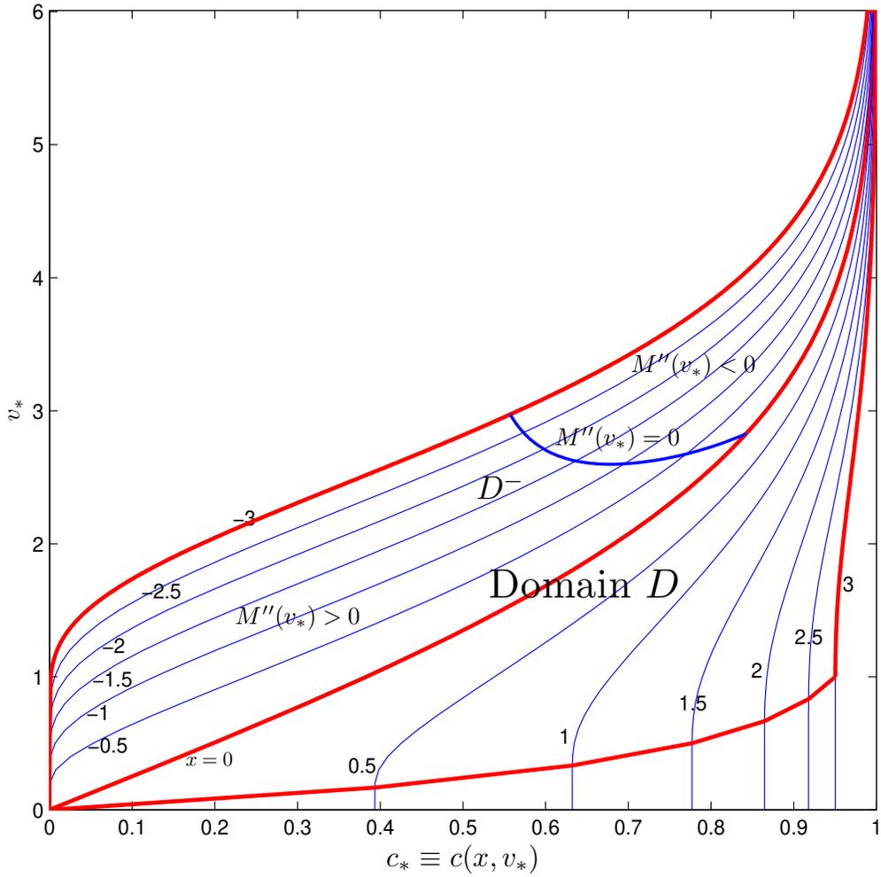
**Figure 5. Domain of inversion  $D$ .**  $D$  is constructed using four criteria, namely,  $0.0005 \leq v_* \leq 6$ ,  $|x| \leq 3$ ,  $0.0005 \leq c_* \leq 0.9995$  and  $|x|/v_* \leq 3$ . Because of the “in-and-out” duality, only options with  $x \leq 0$  will be considered. The curve  $M''(v_*) = 0$  divides the left half domain  $D^-$  further into two parts.
