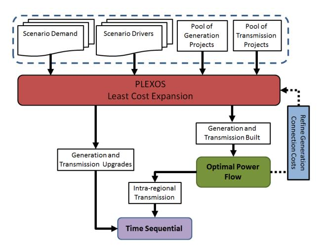
Figure 2: PLEXOS Least Cost Expansion Modelling Framework
