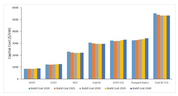
Figure 16: Technology Costs for Conventional Electricity Generation
