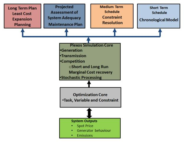
Figure 1: PLEXOS Simulation Core
