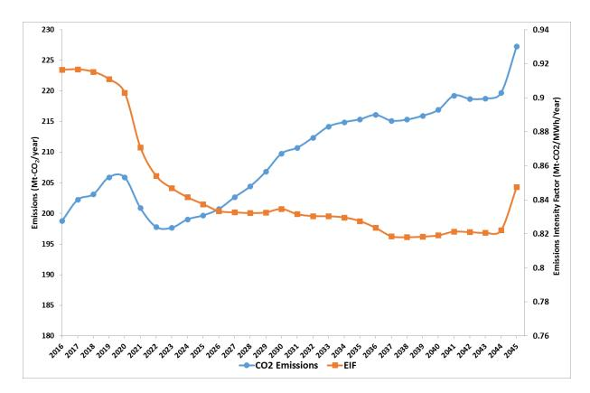
Figure 23: Carbon Emissions due to combustion in Scenario 1
