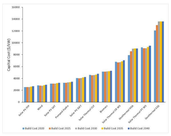
Figure 17: Technology Costs for Renewable Electricity Generation
