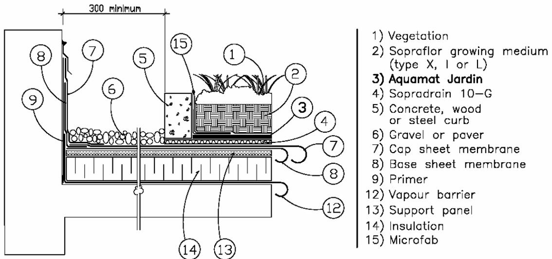
The Soprema system is typically used with its proprietary waterproofing membrane. The Hydrotech system is essentially similar in concept to the Soprema system, but also uses its own proprietary roofing membrane.
