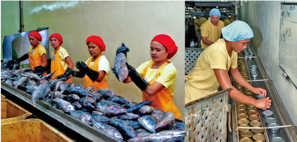
Figure 9.3. Can Filling and Classifying in RDEX Food International Phils Inc
