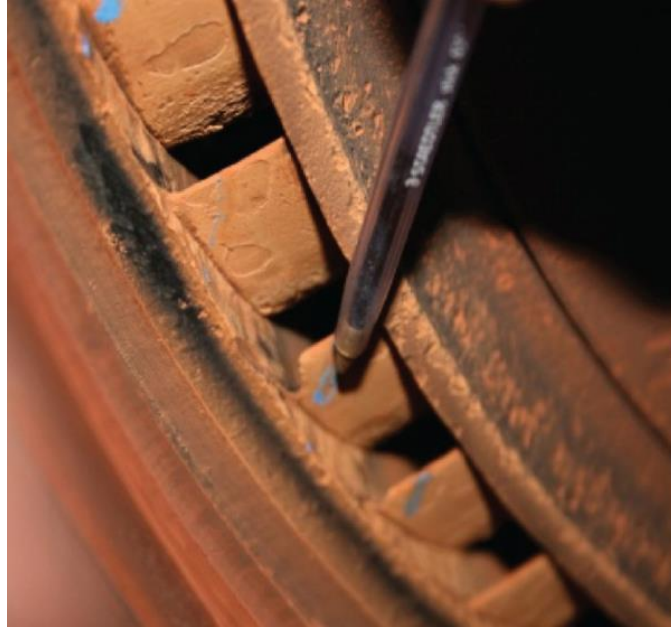
Figure 3-d Corrosion causes imbalance. Failure of this high-pressure rotor control stage was caused by uneven distribution of steam due to corrosion [6].
