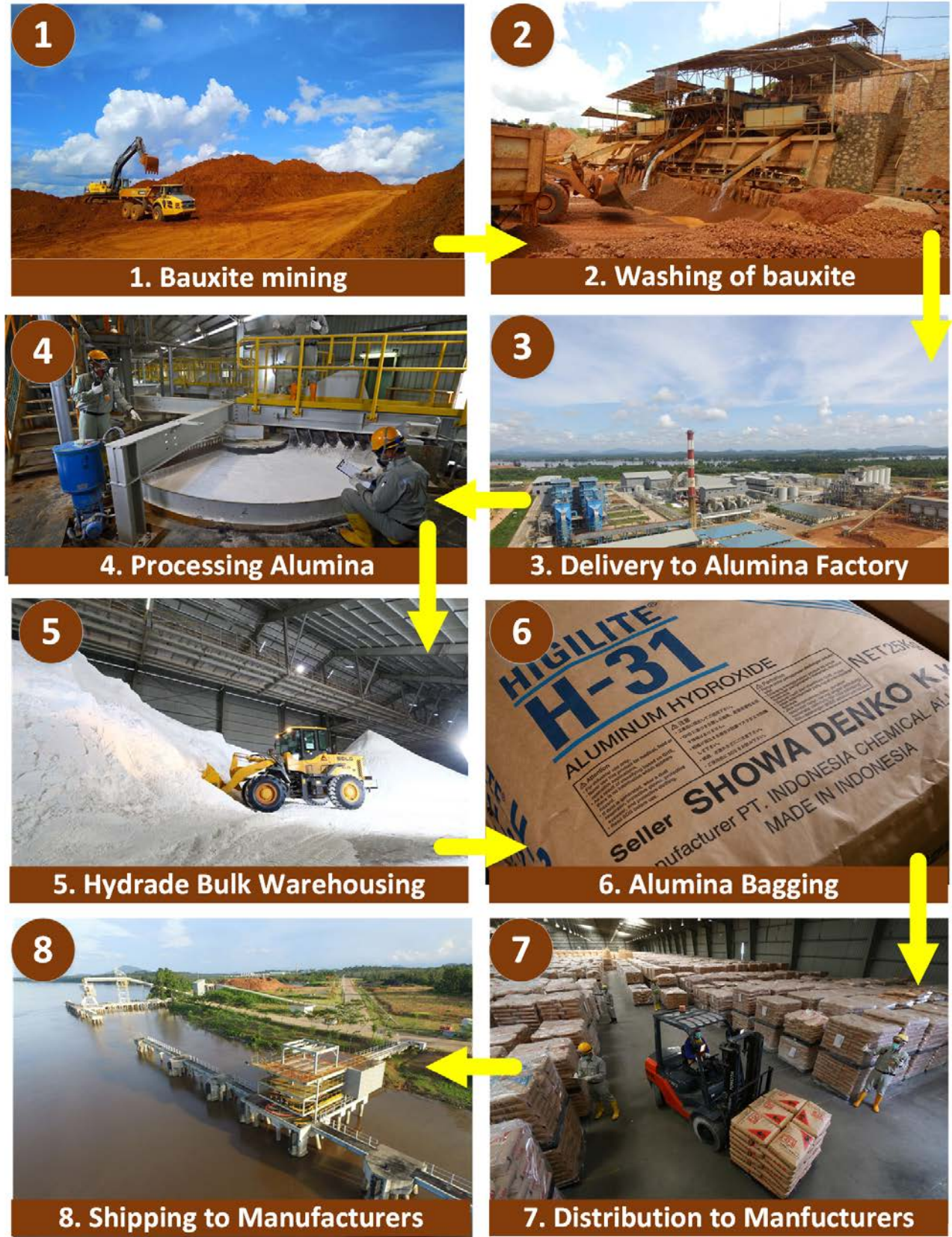
Figure 9.5. Steps in Alumina Factory Processing
