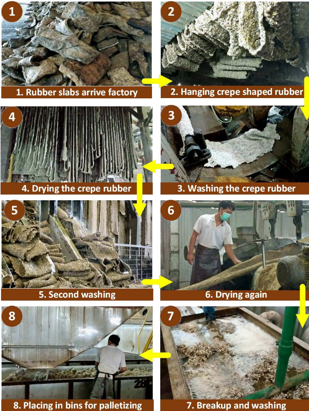
Figure 10.3. Steps in Natural Rubber Factory Processing
