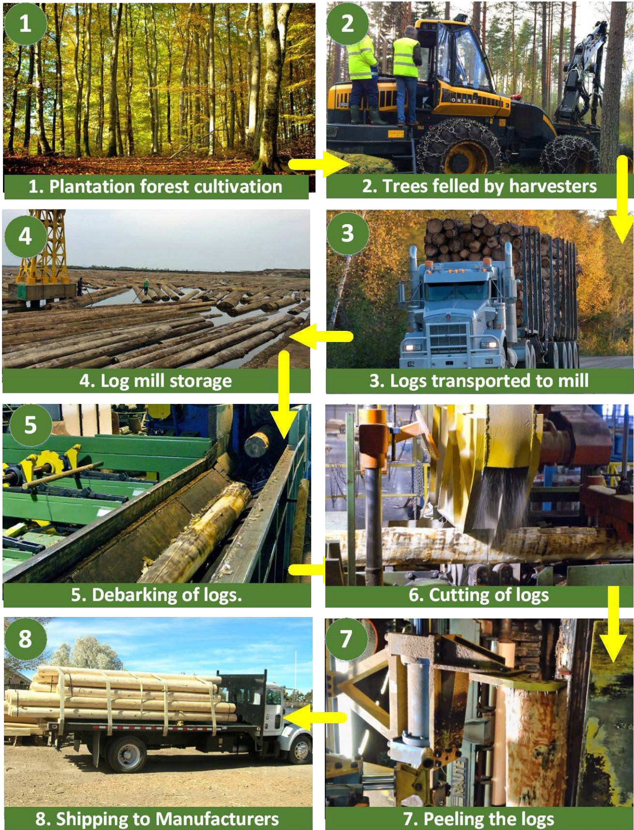
Figure 12.5. Steps in Modular (Knockdown) Furniture Manufacturing
