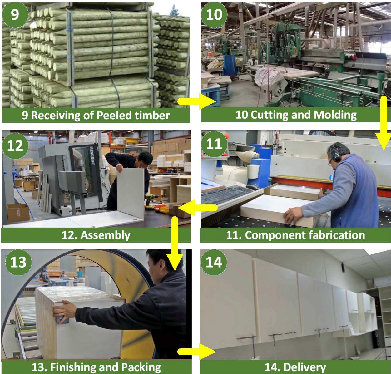
Figure 12.5. Steps in Modular (Knockdown) Furniture Manufacturing (Continued)
