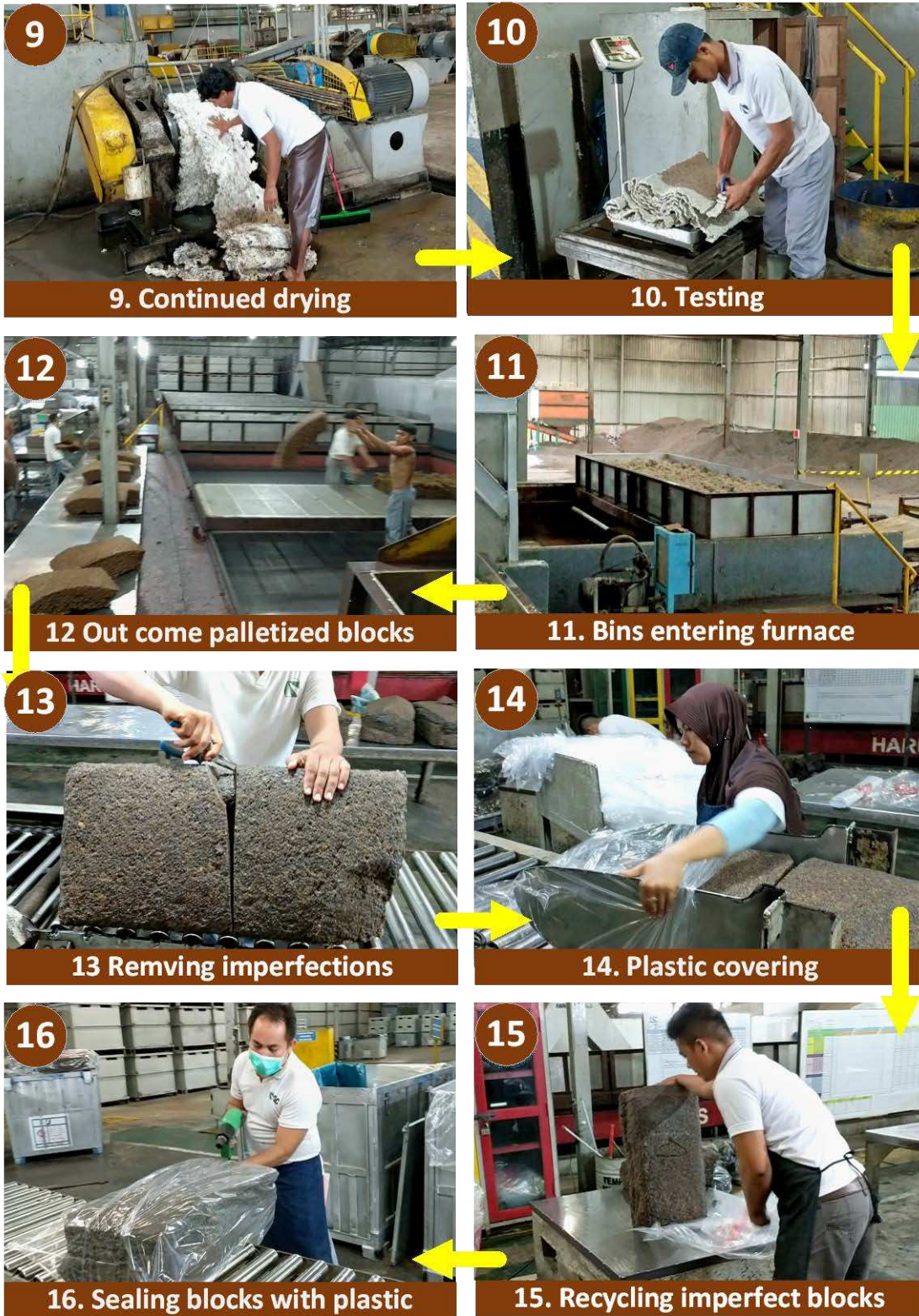
Figure 10.3. Steps in Natural Rubber Factory Processing (Continued)
