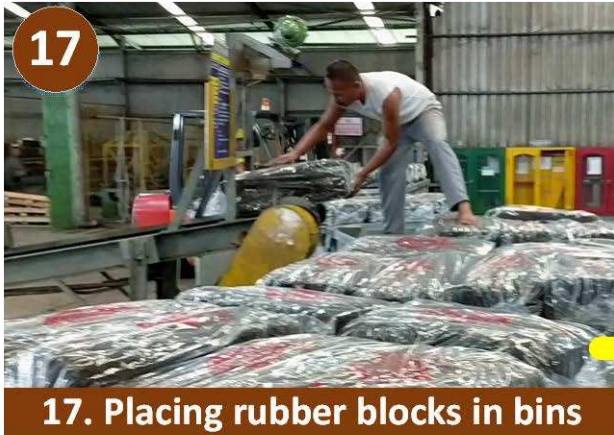
Figure 10.3. Steps in Natural Rubber Factory Processing (Continued)
