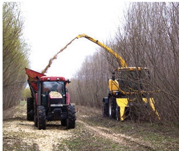
Figure 5.12 : Harvesting willow with a one-pass cut and chip forage harvester
