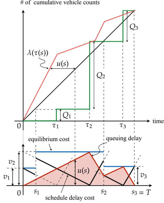
Figure 3: Optimal departure flow pattern, cost pattern, and resulting arrival flow pattern ( $K = 3$ )
