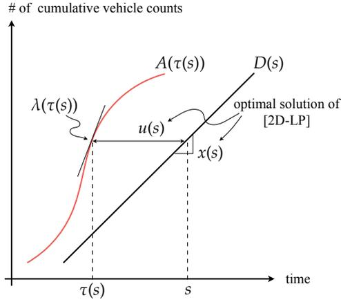
Figure 1: Schematic illustration of construction of cumulative arrival curve from the solution of [2D-LP(x)]
