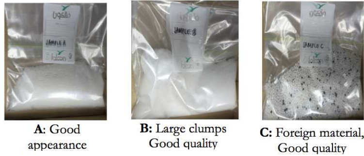
Figure 1: Pictures of samples shown to farmers for the willingness-to-pay assessment. Sample A represented. All three 1 kg samples of urea were purchased as shown by the research team in the market. All three samples were tested by Thornton Labs in the United States and were found to contain 46% nitrogen. Sample A was clean with no caking; Sample B included two large, hard caked aggregates; and Sample C included the presence of foreign material mixed in the urea.
