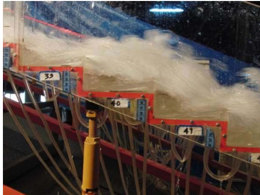
Fig. 11. 10 degrees slope and 30 liter per second flow rate
