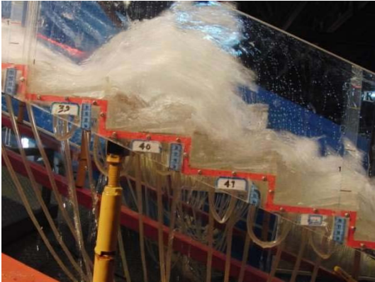
Fig. 5. Figure 4-steps with 7 degrees slope and 6 mm sill's height and 5 mm width
