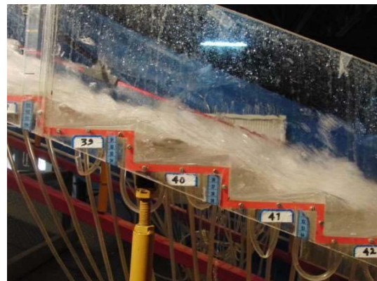
Fig. 9. 7 degrees slope and 30 liter per second flow rate
