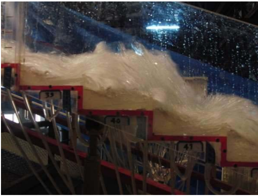
Fig. 4. Steps with 12 degrees slope and 15 mm sill's height and 5 mm width
