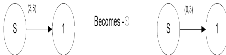
Figure 6.29: An example of subtracting the lower bound from both the upper and lower bounds.
