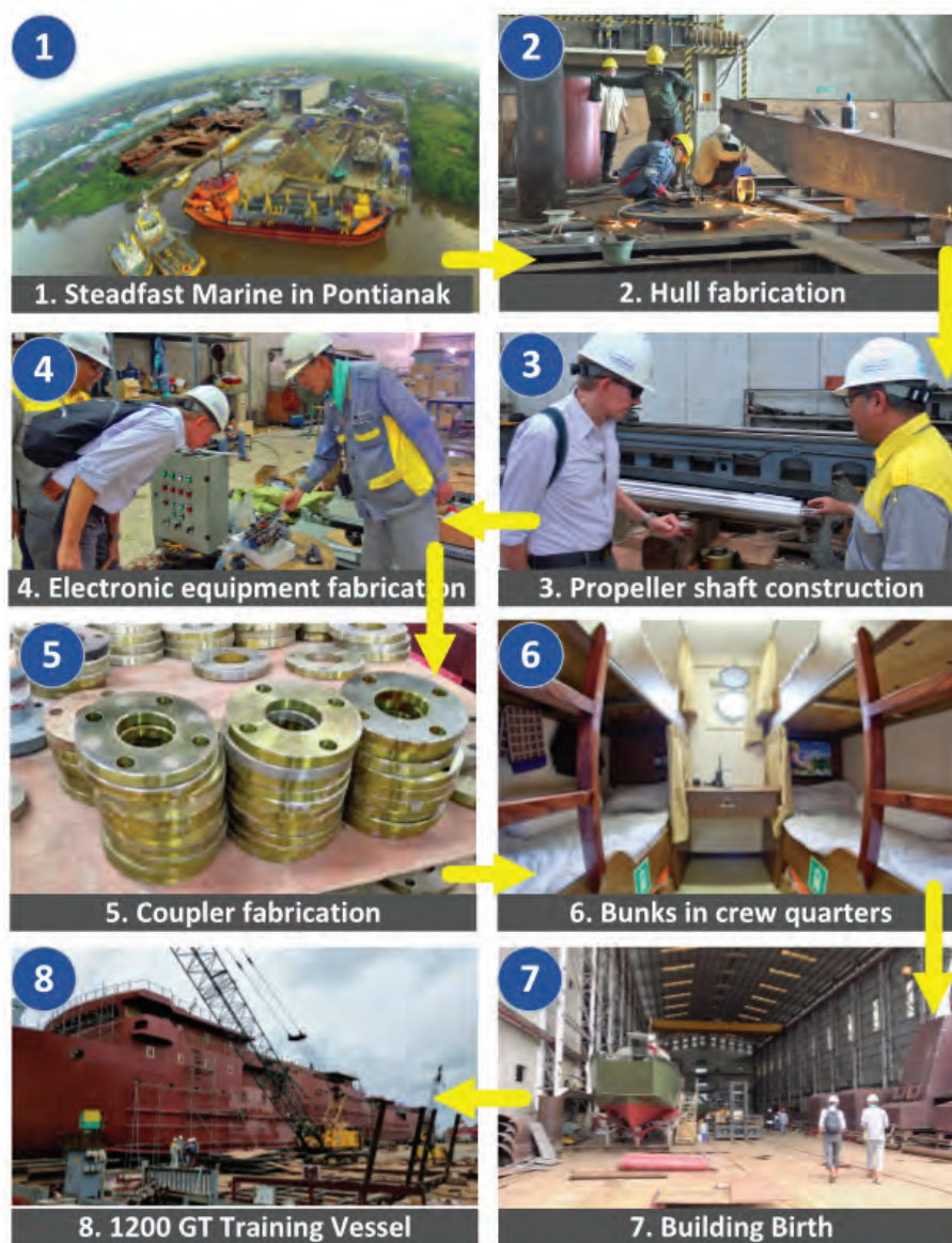
Figure 20.7. Steps in a Shipbuilding Process
