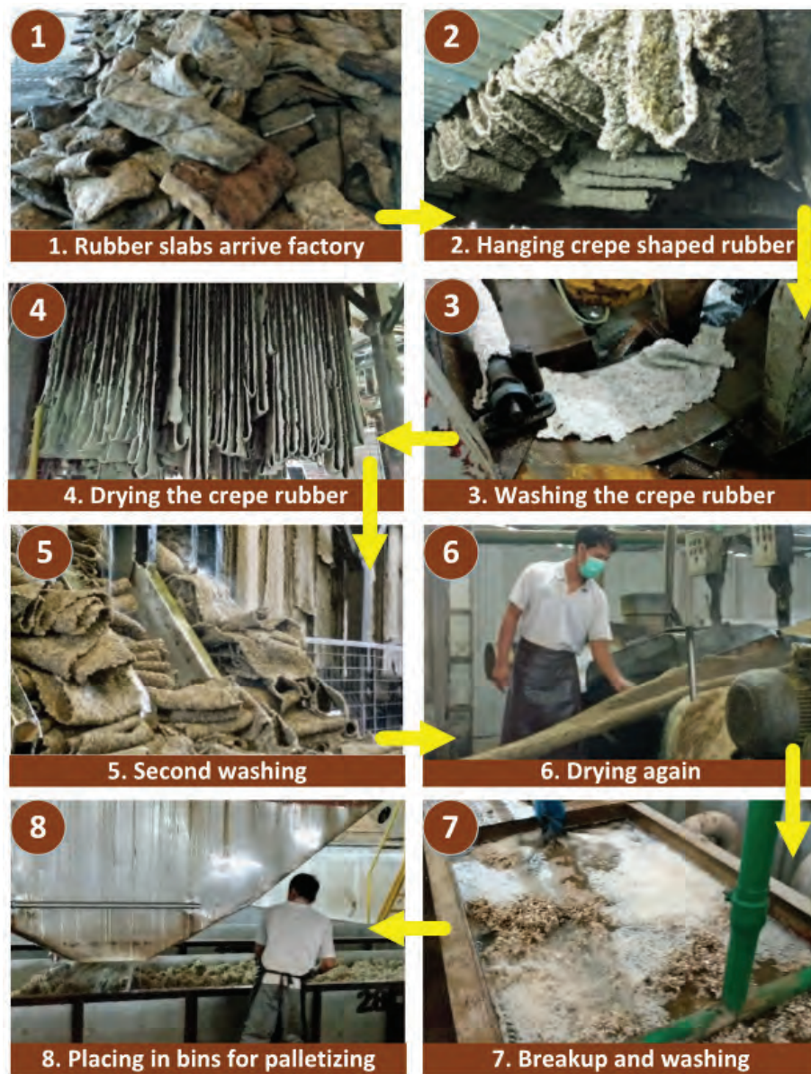
Figure 16.6. Steps in Natural Rubber Factory Processing
